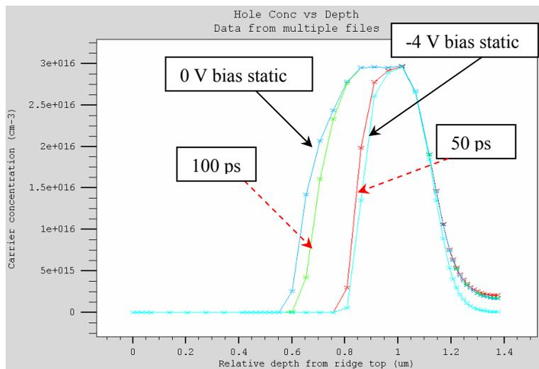
Fig.5 Hole concentration along the vertical bi-sectional line of the waveguide.
