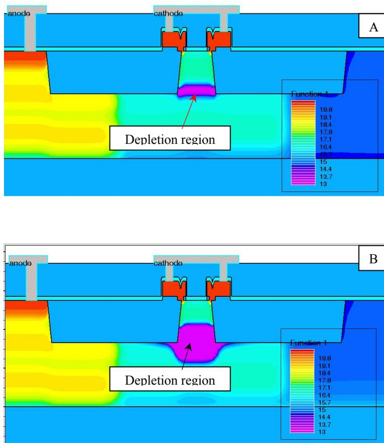
Fig.3 Contour of  $\text{Log}_{10}(\text{electron} + \text{hole concentration})$  showing the depletion region at A) 0 V bias, B)  $-4\text{v}$  bias.
