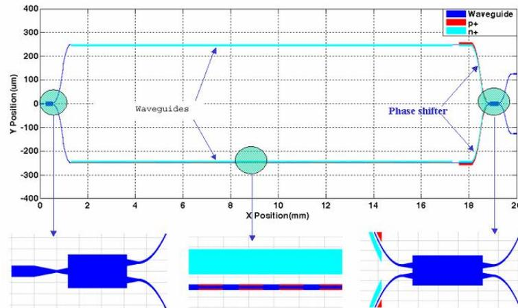
Fig.6 Layout of the MZ interferometer based amplitude traveling wave modulator.
