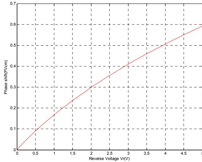
Fig.4 Phase shift per-centimeter-long waveguide versus the reverse bias voltage of the diode.
