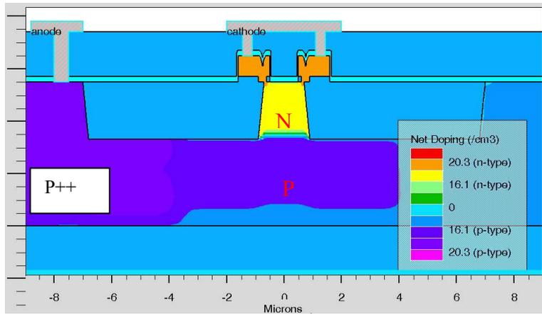
Fig.2 A cross-sectional schematic showing the doping profile and metal contacts.
