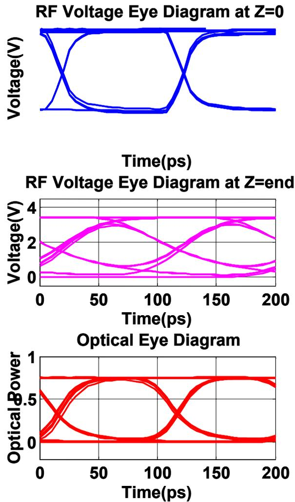
Fig. 8 Electrical and optical eye diagram showing the performance of the modulator, 64-bit pseudo random signal input.
