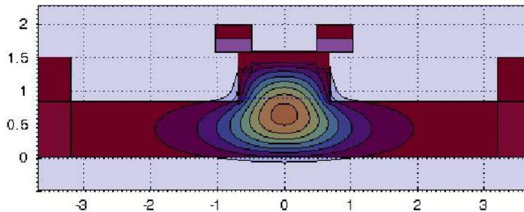
Figure 1. Mode shape of the waveguide
